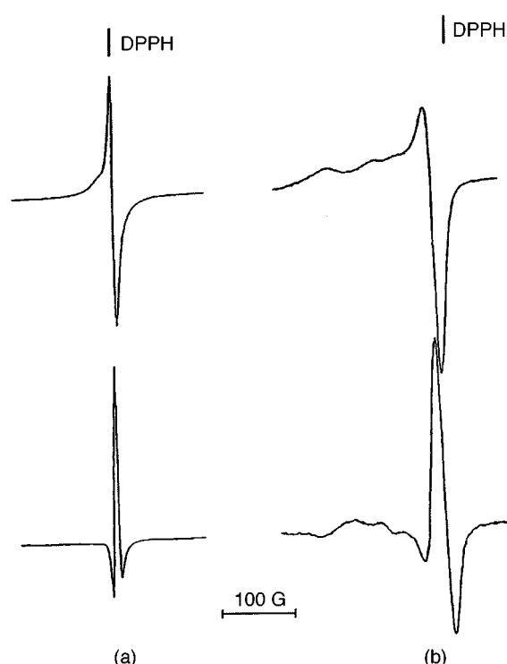
Fig. 3 X-Band EPR spectra recorded at 100 K on CH 2 Cl 2 solutions of: (a) [C 60 ] − ; (b) [1] − . Top: first derivative mode; bottom: second derivative mode.
